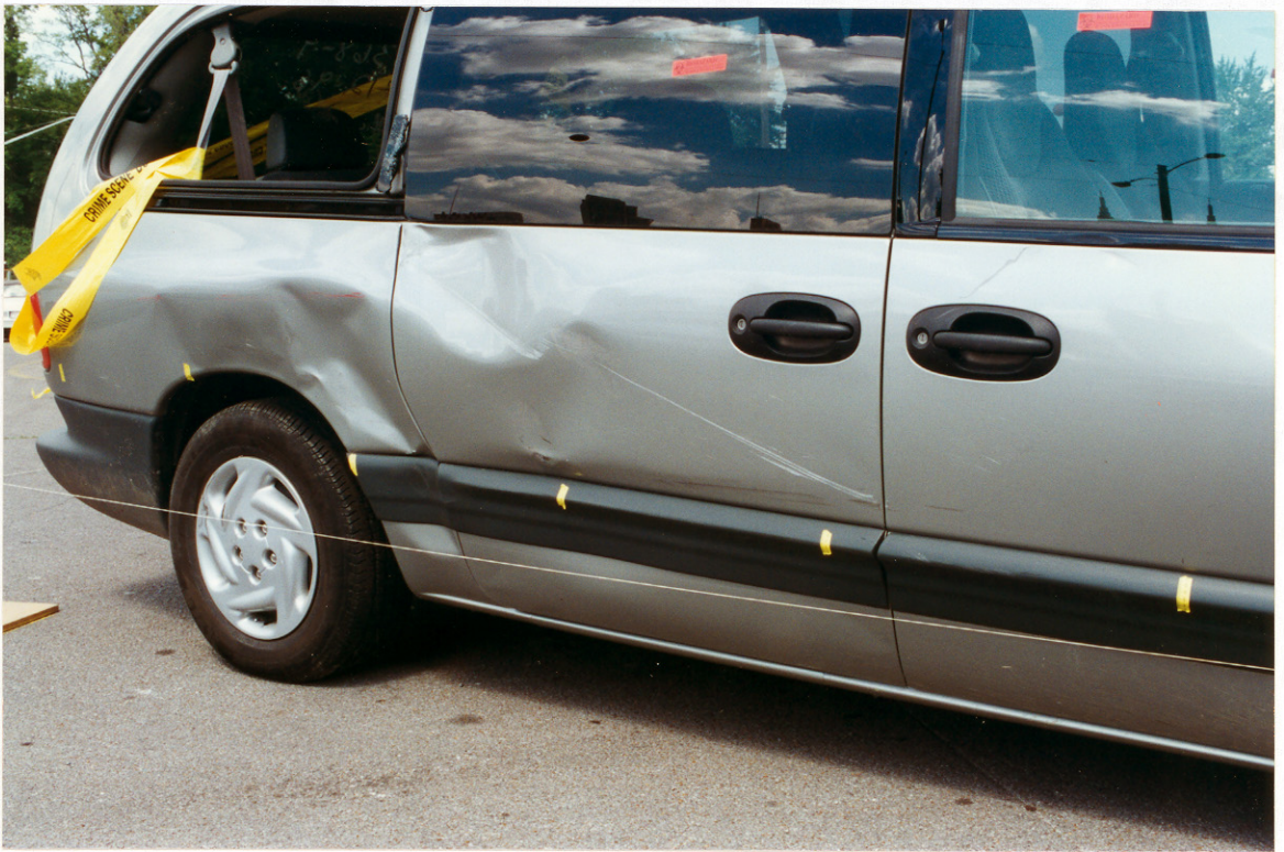
44. Right rear side slap damage to the Dodge Caravan.
